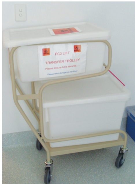
Specific transfer trolley used in CSIRO to transfer LMO and related materials
