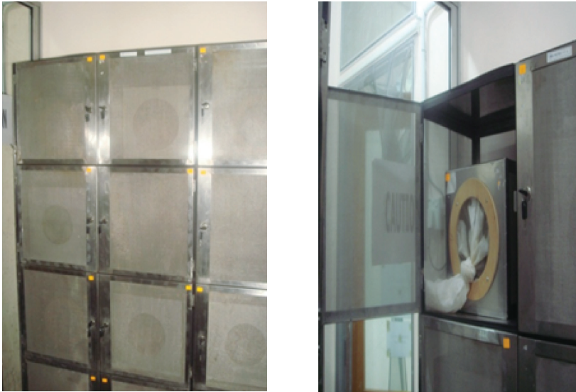
Arthropod cages constitute the primary containment in insectariums. Adult mosquitoes kept in rearing cages. Access is via a 60cm long cloth sleeve (surgical stockinet) that fits an opening on 1 side of the cage. The cages are kept in ventilated secure cabinets. (Source: IMR)
